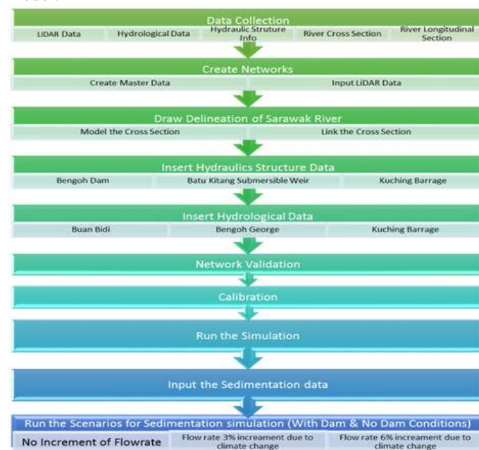
Fig.2: Flowchart for sedimentation simulation using Infoworks RS
